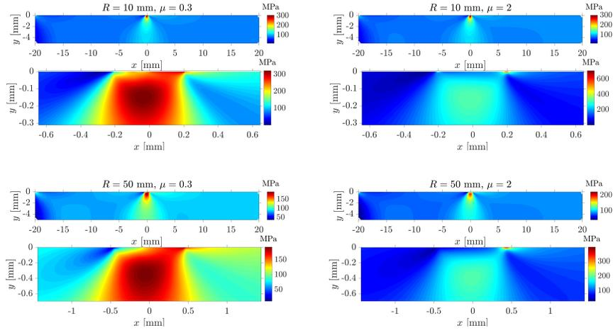
Figure 4: Von Mises stress of four considered cases computed by MLSM on densest meshes. In each panel, a stress in a whole specimen is shown on the top, followed by a magnified picture showing only the region under the contact area.
