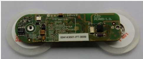
Figure 2. Prototype of the wireless multifunctional body sensor
