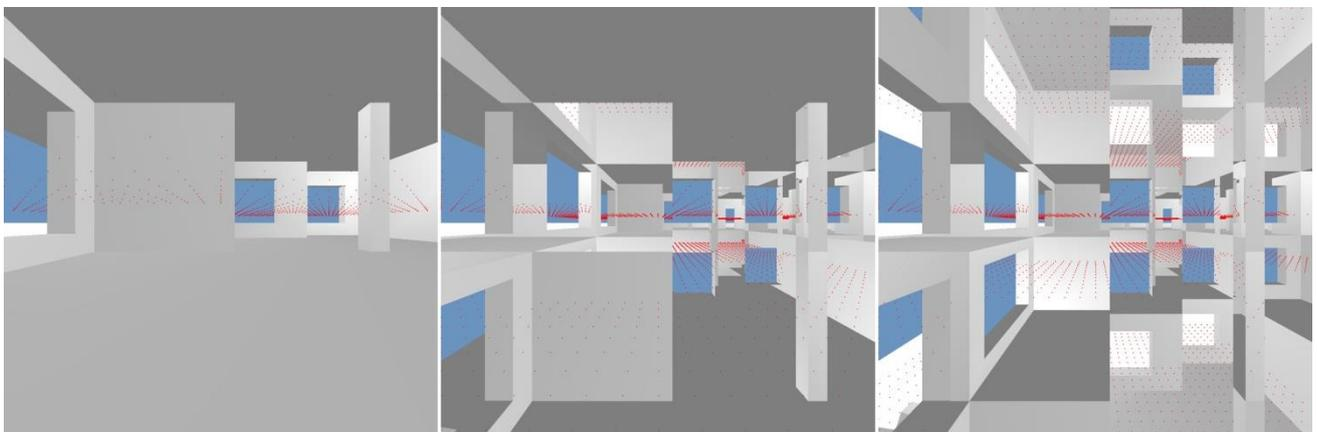
Fig. 3 Radio signal reflections and double refractions are recursively traversed using graphic primitives. The illustration shows three snapshots of a framebuffer object at increasing tree depths. Color-coded surfaces are replaced by black-and-white rendering of scene objects with visible reception points superimposed as red dots.
