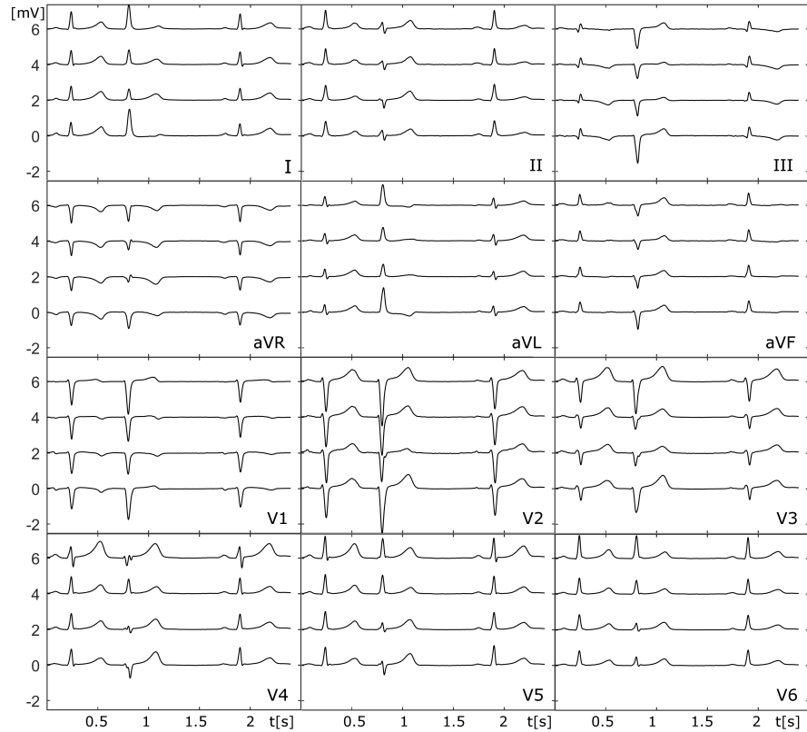
Fig. 5.5 Target 12-lead ECG (the bottom curve in each panel) and three synthesized 12-lead ECGs (the curves moved up by 2, 4 and 6 mV) drawn in this bottom-up order: (I) personalized DL positions and personalized transformation, (II) universal DL positions and personalized transformation, (III) universal DL positions and universal transformation. The second beat is an extrasystole.
