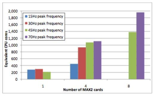
Figure 1: Performance of Maxeler-accelerated Finite Difference Modeling, using a large scale system based on MAX2 cards. Source: [Oriato2010]
