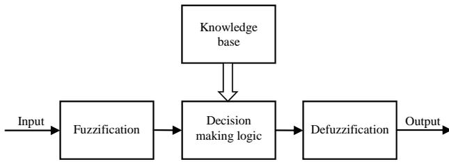
Fig. 3. Block diagram of a fuzzy logic controller.
