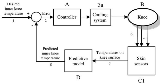
Fig. 2. Schematic diagram of the feedback control loop.
