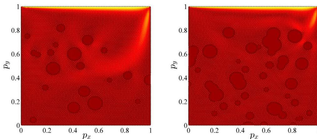
Fig. 12. Solution of lid driven problem in a domain filled with randomly distributed circular obstacles: left 20 obstacles, right 50 obstacles.
