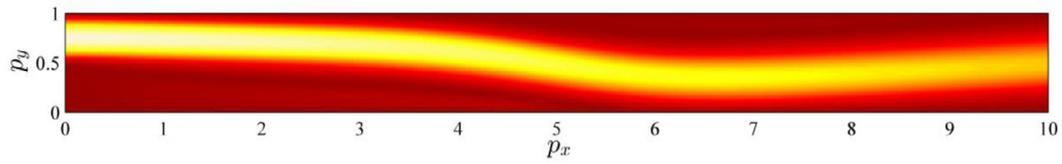
Fig. 6. Velocity magnitude contour plot for backward-facing step problem.
