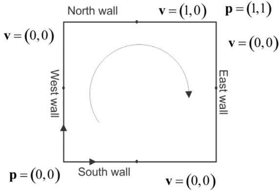
Fig. 2. Scheme of the lid driven cavity problem.
