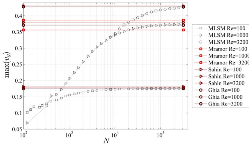
Fig. 5. The maximal mid-plane velocity  $\max(v_y(p_x, 0.5))$  with respect to the number of computational nodes for different Re numbers. Blue, black and green lines stand for reference solutions *Mramor*, *Sahin* and *Ghia*, respectively. (For interpretation of the references to colour in this figure legend, the reader is referred to the web version of this article.)
