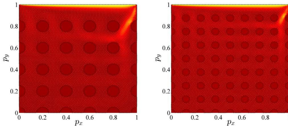
Fig. 11. Solution of lid driven problem in a domain filled with uniformly distributed circular obstacles: left 30 obstacles, right 72 obstacles.
