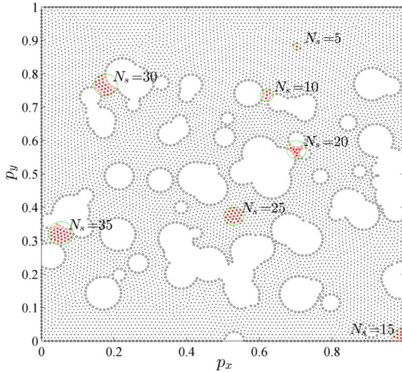
**Fig. 1.** Distribution of nodes within a randomly generated domain. The example support domains nodes are marked with red circles. (For interpretation of the references to colour in this figure legend, the reader is referred to the web version of this article.)
