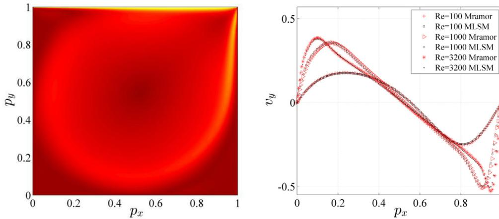
Fig. 4. Contour plot of velocity magnitude for Re=3200 (left) and comparison of horizontal mid-plane velocity profile  $v_y(p_x, 0.5)$  against recently published solution *Mramor*.
