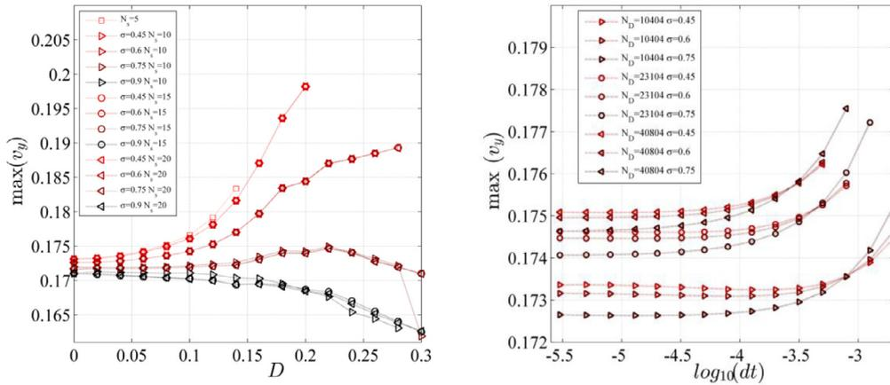
Fig. 9. The impact of nodal deformation on the performance of the method with respect to the support domain size and weight parameter (left) and the impact of the time step, weight parameter and number of computational nodes on the results (right).
