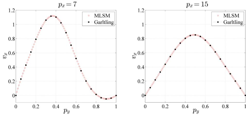
Fig. 7. Comparison of vertical velocity profiles at  $p_x = 7$  and  $p_x = 15$  for backward-step facing problem.
