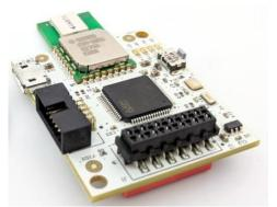
Fig. 2 IR-UWB board with DWM1000 was developed in order to address low cost sensor node localization problem.
