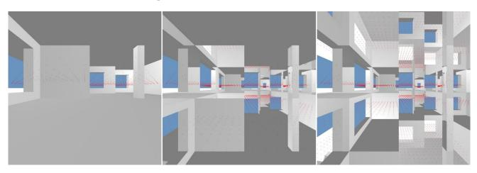
Fig. 3 Radio signal reflections and double refractions are recursively traversed using graphic primitives. The illustration shows three snapshots of a framebuffer object at increasing tree depths. Color-coded surfaces are replaced by black-and-white rendering of scene objects with visible reception points superimposed as red dots.
