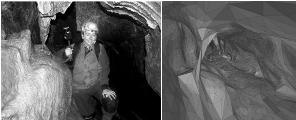
LiDAR Survey Exercise in Skirwith Cave using ZEB1 and 3D Model of cave
